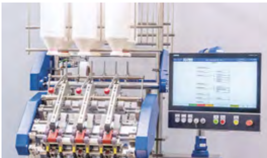
The LSE 2000-2 is designed for processing staple fibers made of cotton, wool, man-made fibers and their blends.
