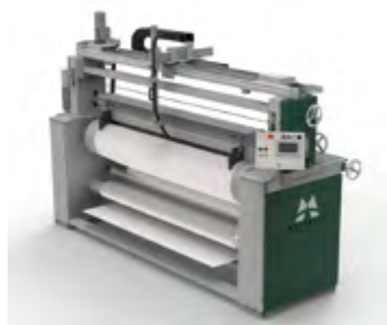
The Coattex coating unit is dedicated to air knife and knife-over-roller coating.
