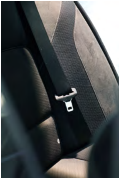
Seat belts must be able to withstand tensile forces of more than 3 tons.
