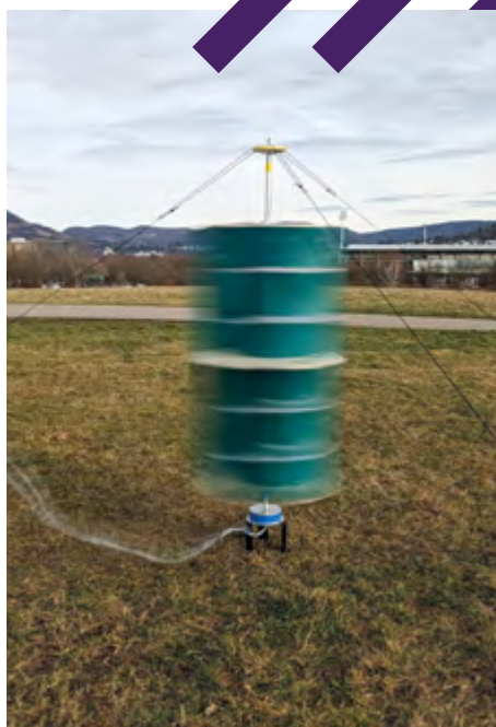
The wind turbine design features a foldable textile rotor.
