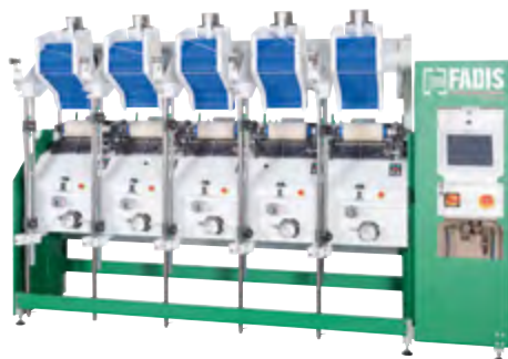
The new machine range guarantees high performance and speeds up to 1,400 m/min.
