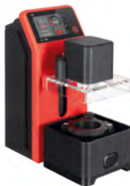
The TSA measures individual components like thermo-haptic, friction, crumple, or drape behavior.
